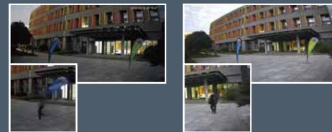
When the light is insufficient, the moving objects are prone to smearing and blurring on the conventional IP cameras.
