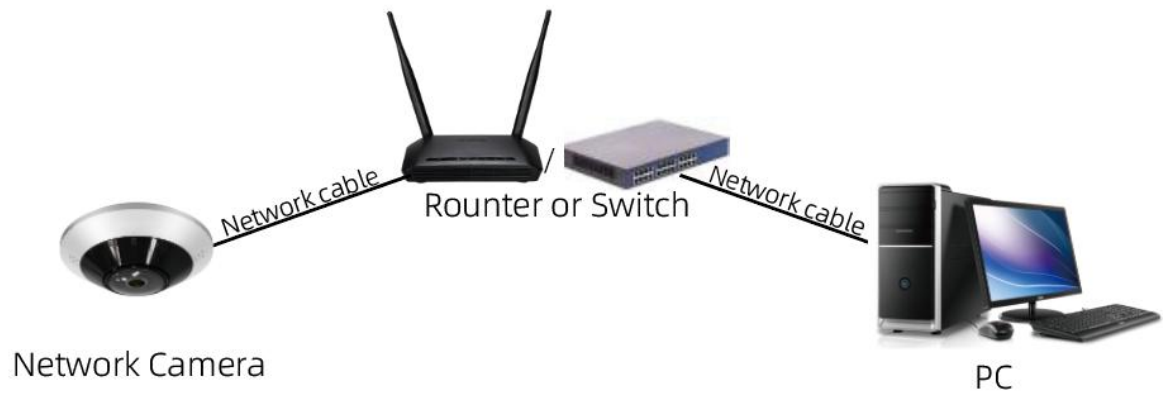
Figure 1-2-2 Connecting via a Switch or a Router
