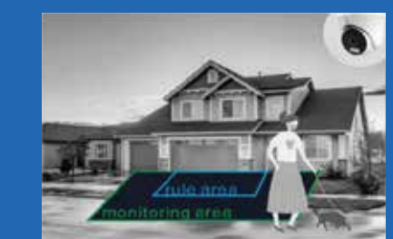
Warm light turns off, IR illuminator turns back on when the target disappears to reduce light pollution.
